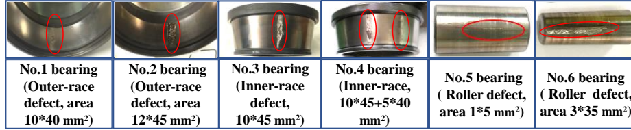
Fig. 2. Faulty bearings.
